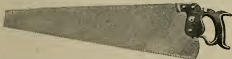
Fig. 87—The Common Grades of both Handsaws and Ripsaws are Made this Shape
